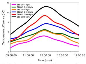
Fig. 6. Time-dependent variation of temperature difference values
