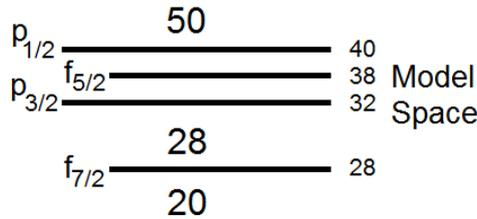
**Fig 1.** Single particle orbits in model space above  $^{40}Ca$  core considered in the calculations
