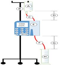
A: Refillable serum bag, B: Serum hanger, C: IV set, D: Fixed distance (30 cm) between serum bag and pump, E: Volumetric infusion pump, F: IV set, G: Fixed distance (80 cm) between pump and graduated cylinder, H: Graduated cylinder.
