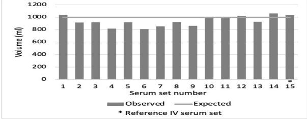
ml: milliliters, Observed: The volume of fluid infused within an hour period by the volumetric infusion pump, Expected: Expected volume of fluid infused within an hour period by the pump, \*Reference IV serum set: Serum set (15<sup>th</sup>) which is an appropriate product for infusion pumps.
