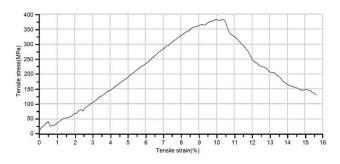
Figure 14 Stress-strain curve of AV sample
