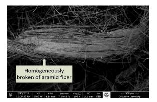
Figure 22 AV composites SEM micrograph
