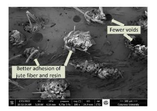
Figure 24 JP composites SEM micrograph
