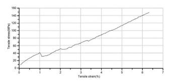
Figure 16 Stress-strain curve of JAV sample
