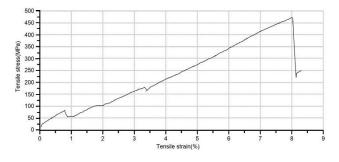
Figure 15 Stress-strain curve of AP sample
