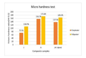
Figure 20 Micro hardness test results
