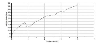
Figure 13 Stress-strain curve of JP sample
