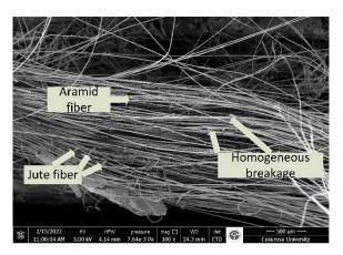
Figure 26 JAP hybrid composites SEM micrograph
