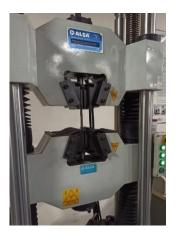
Figure 6 Tensile testing machine
