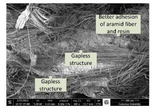
Figure 25 AP composites SEM micrograph
