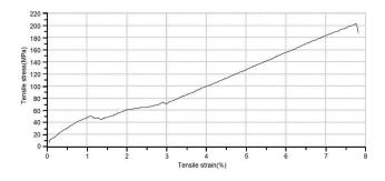
Figure 17 Stress-strain curve of JAP sample
