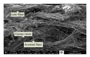
Figure 23 JAV hybrid composites SEM micrograph
