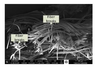
Figure 21 JV composites SEM micrograph
