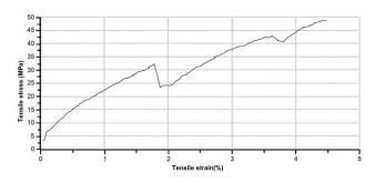
Figure 12 Stress-strain curve of JV sample
