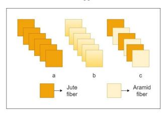
Figure 3 Fabric stacking sequences of a) JP b) AP c) JAP
