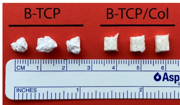
**Figure 1.** Image of B-TCP (SupraBone, 0.5–1mm particle size) and Image of B-TCP/Col (0.5 mm x 0.5 mm x 0.5 mm).
