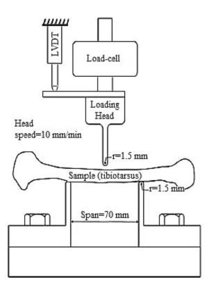
Figure 1. Schematic presentation of three-point bending test on tibiotarsus (modified from Suzer et al.26)
