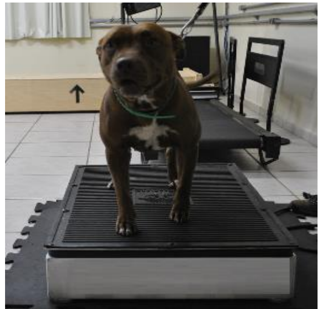
Figure 1. Dog standing on the top of the vibrating platform which delivered a vortex wave circulation, and with a leash to prevent from moving or sitting.
