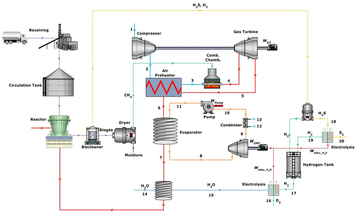
Figure 2. The operating principle of the Afyon biogas plant.
