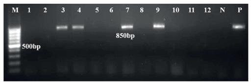
**Figure 2.** Agarose gel image of PCR-amplified DNA bands of coat protein gene of BCMV isolates M: 1kb DNA marker (Thermo Scientific), P: Positive control, N: Negative control, Lane 3, 4, 7, 9: BCMV-infected bean samples.
