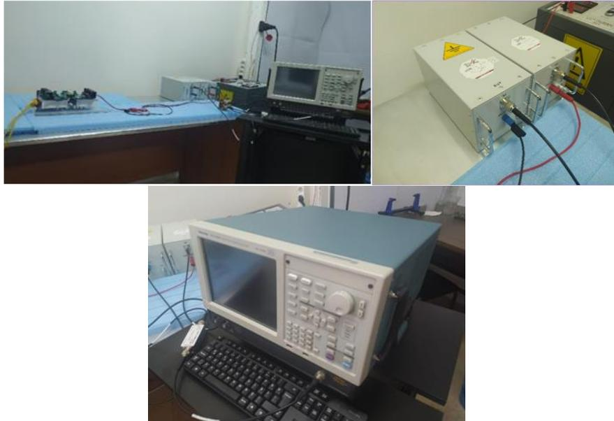
**Figure 9:** Conducted Emission Lab Test Bench, LISN and Spectrum Analyzer
