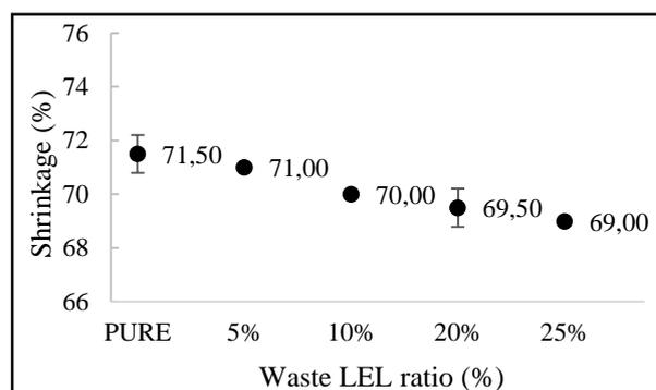
**Figure 14.** Graphical representation of shrinkage values of LEL films
