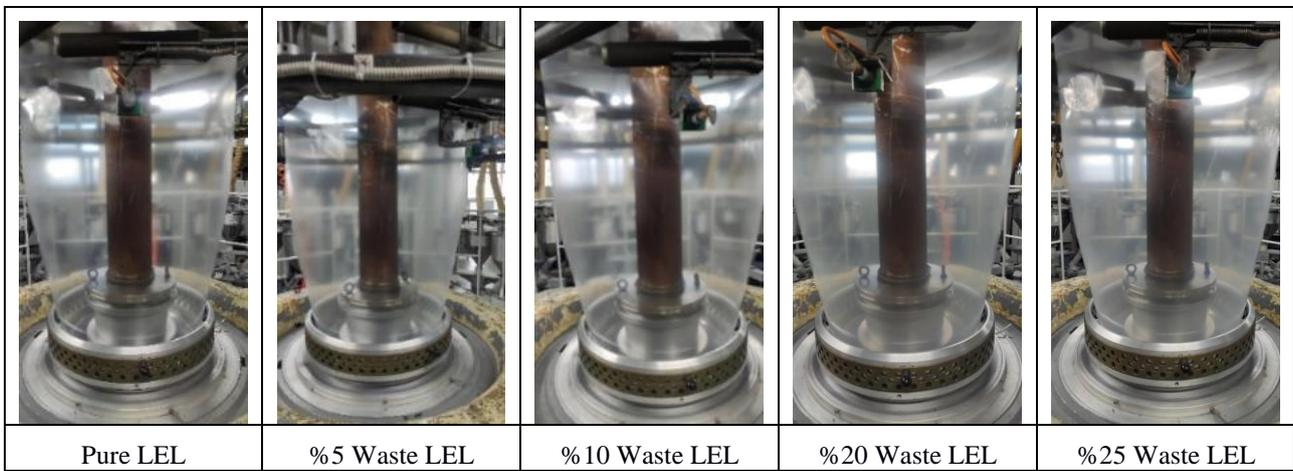
**Figure 2.** Output of films with different waste LEL ratio from the extruder heat
