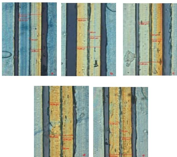
**Figure 15.** Microscopic views of LEL films formed with waste EVOH and LDPE a) Pure LEL, b) 5% waste LEL,
