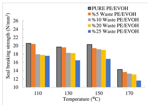
**Figure 12.** Graphical representation of seal breaking strength values of LEL films
