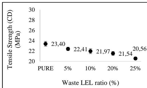
**Figure 4.** Graphical representation of CD tensile strength values of LEL films
