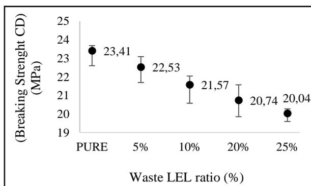
**Figure 6.** Graphical representation of the CD breaking strength values of LEL films
