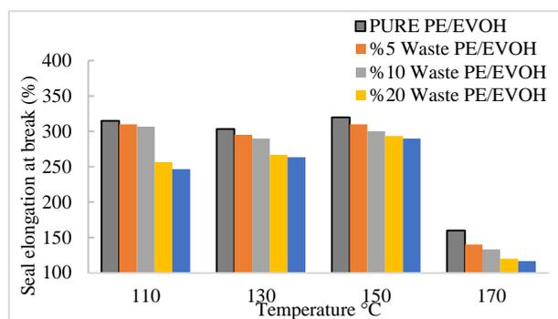
**Figure 13.** Graphical representation of seal elongation at break values of LEL films
