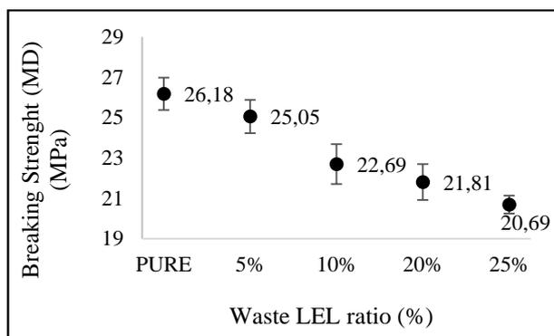
**Figure 5.** Graphical representation of the MD breaking strength values of LEL films
