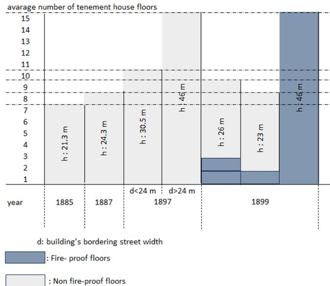
**Figure 12.**The maximum building height criteria based on the width of the facade and fire-resistant floor design (drawing by authors)
