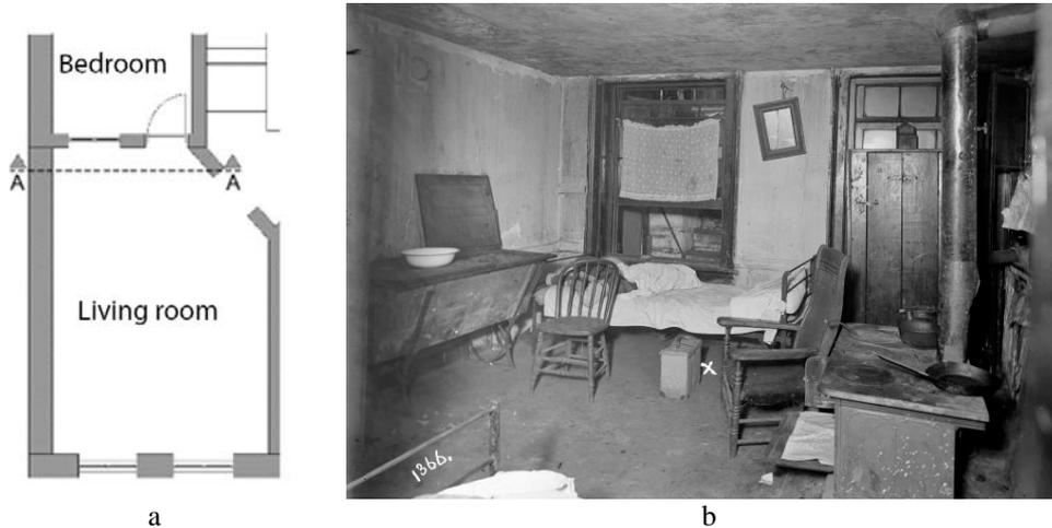
**Figure 6.** (a) Window plan opening from dark inner rooms to the living room (drawing by authors), and (b) Minimum 30 cm<sup>2</sup> opening above the door and minimum 0.90 m<sup>2</sup> window opening from the dark room to the front room (URL-4)
