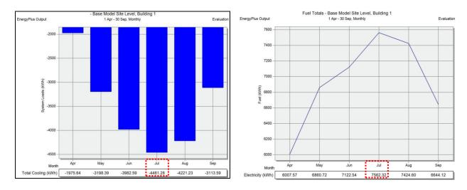
*Figure 20.* Total cooling load result after applying all proposed passive cooling techniques
