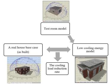
*Figure 3.* A diagram shows the methodology steps of the energy simulation process and the scenarios of each phase
