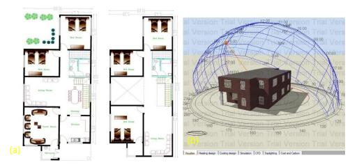
*Figure 13.* (a) Two dimensional drawing of the energy simulation by using AutoCAD, (b) 3d view of the actual house modeled using DesignBuilder
