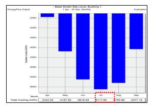
*Figure 17. Total cooling load result after applying Mahrabyiya covering the exterior windows*
