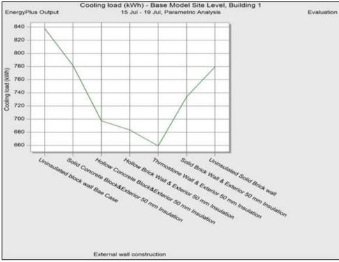
*Figure 10.* Comparative simulation analysis of all proposed wall thermal mass with exterior insulation in relation with cooling load calculation
