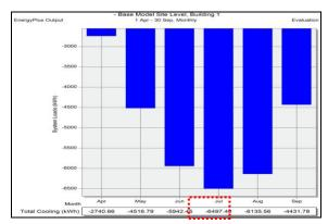
*Figure 18. Total cooling load result after applying Mahrabyiya to cover the flat roof*
