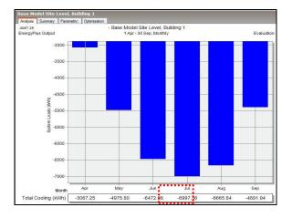
Figure 14. Total cooling load performance of the base case house during summer from April to September showing the peak cooling load in July
