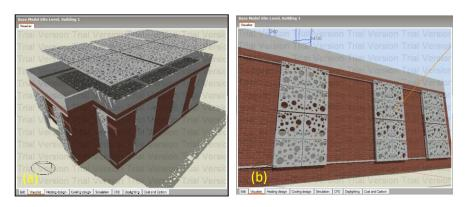
Figure 16. The proposed movable Mashrabiya screen as external shading device of roof (a) and windows (b), modeled by using DesignBuilder
