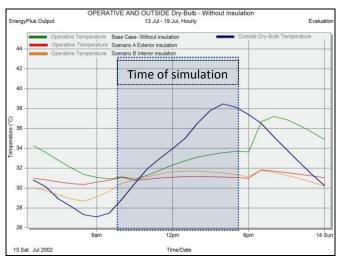
Figure 11. Simulation results showing the effect of all roof thermal insulation scenarios on indoor operative temperature
