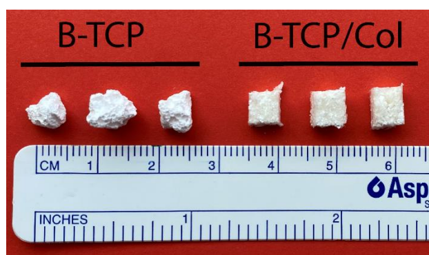
Figure 1. Image of B-TCP (SupraBone, 0.5–1mm particle size) and Image of B-TCP/Col (0.5 mm x 0.5 mm x 0.5 mm).
